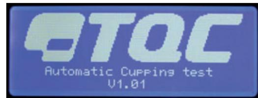
After a few seconds the time and date screen appears showing the time left till next calibration. When a calibration is required the TQC Automatic cupping test will inform the user that calibration is required in this screen. The linguistical warning is also accompanied with audio warning.
