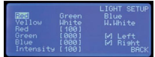
The intensity setting lets you set the strength of the light. The left and right check boxes allow you to set the direction of the light. Cracks can best be seen when the complementary colour to the test panel is used to illuminate the panel .
