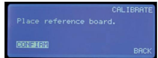
The TQC Automatic Cupping test now starts to search for the calibration plate. By slowly moving the indenter towards the plate. This can take several seconds for the calibration to be finished. While the calibration is in progress 'Calibrating reference....' is shown.
