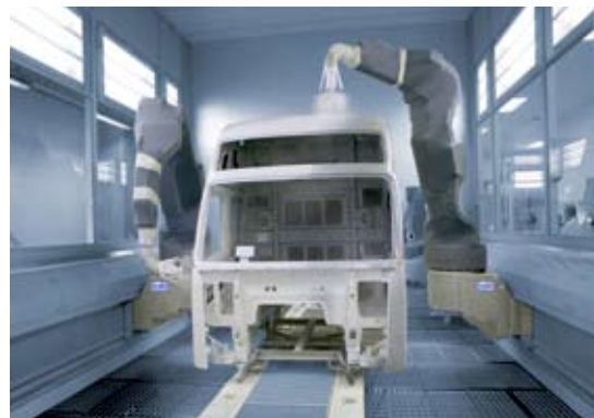
EcoBell2 SL Atomizer used in production for painting driver's cabs
