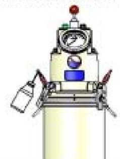
6. While the water is flowing constantly, tip the unit on its side and rotate it in circular motion until the water flows out of the right ball shut-off valve without bubbles.
