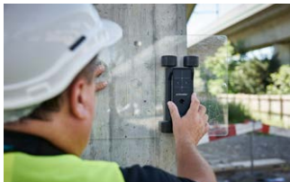
Figure 33: Scanning near to the edge
