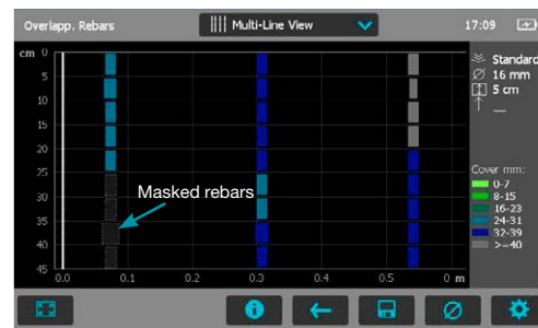
Figure 23: Multi-Line View with masked rebars
