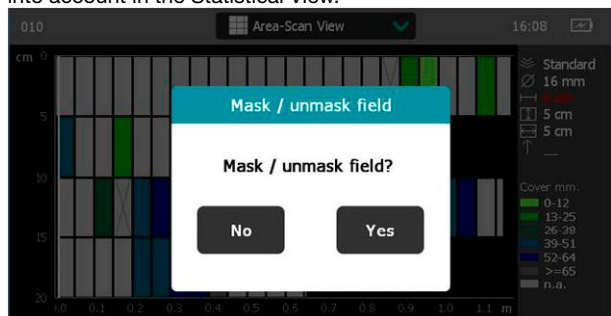
Figure 15: Area-Scan option to mask a field by double-tapping on it
