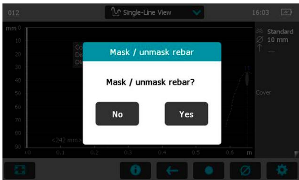
Figure 12: Single-Line option to mask a rebar by double-tapping on it
