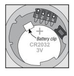
down. Replace both batteries, positive side up, replace cover.
